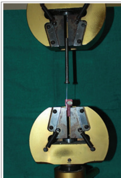
Figure 7. Showing test unit attached to INSTRON for frictional resistance measurement
