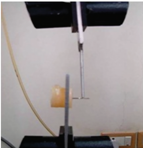
Fig. 3: Cast clasp mounted on universal testing machine
