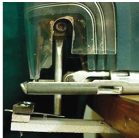
Fig. 4: Closeup of cast mounted on custom-made oscillation machine (Black and Decker)
