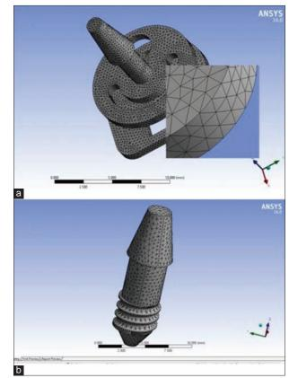
Figure 2: (a) Meshing of disc implant, (b) Meshing of screw implant
