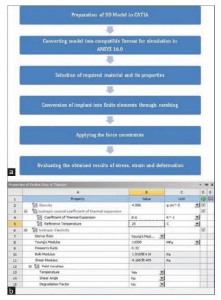
Figure 1: (a) Flowchart of methodology, (b) Material specification module in ANSYS 16.0
