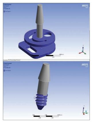
Figure 3 : Supporting the surfaces of implants
