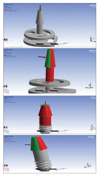
Figure 4: Application of forces on selected surfaces
