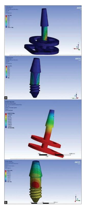
Figure 5: (a) Stress values and its distribution, (b) Deformation of implant (Simulation)
