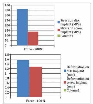
**Graph 1:** Graph showing amount of stress and deformation on disc and screw type of dental implant
