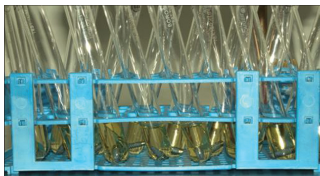
Figure 6: 15 assembled implants and abutments dropped in sterile brain–heart infusion broth
