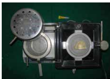
Figure 5. Biostar moulding machine wherein Bioplast material is moulded on upper model with acrylic blocks and incorporated into wire component.
