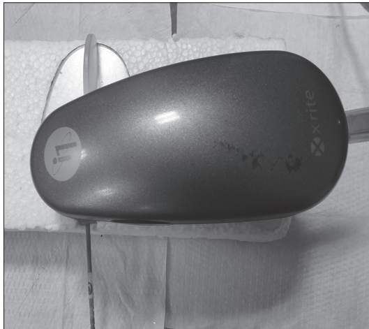
Figure 2: Use of X-Rite i1Pro reflectance spectrophotometer for color evaluation
