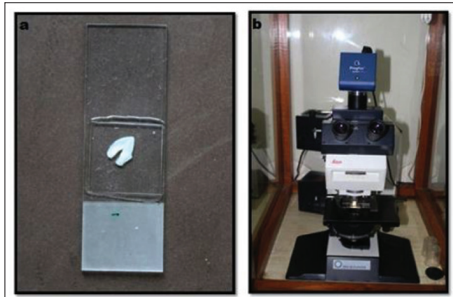
Figure 4. (A) Mounting Done on Glass Slides Using Mountant (b) Polarized Light Microscope (Leica DMRB, Germany)
