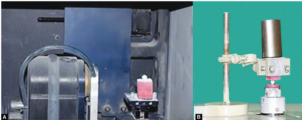
Figs 3A and B: (A) Extracted tooth placed inside the extraoral laboratory scanner; (B) Extracted tooth placed onto the upper holder while disc sample was placed on the lower holder of a two-body wear machine
