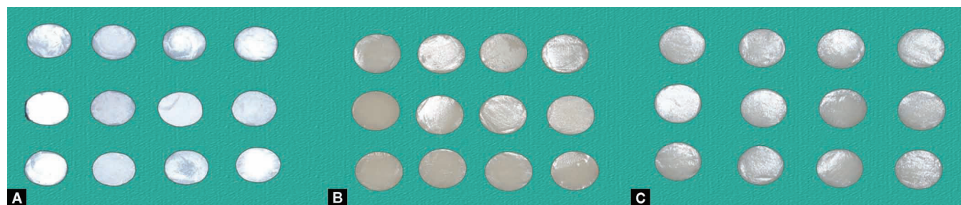
Figs 1A to C: Milled discs measuring 10 \times 2 mm: (A) Zirconia; (B) Resin nanoceramic; (C) Polymer infiltrated ceramic network
