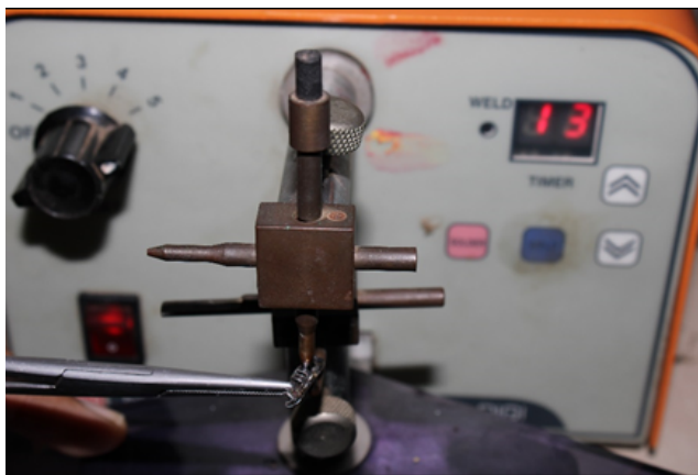
Fig. 2: Welding palatal sheath with band material
