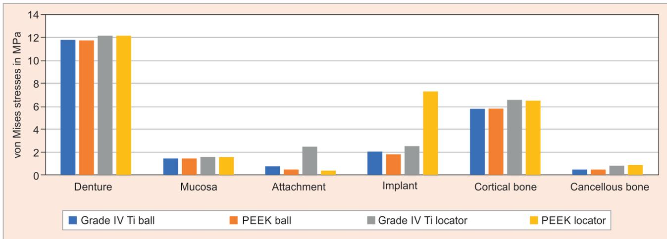
Fig. 6: Comparison of VMS generated with tripod ball and locator attachments
