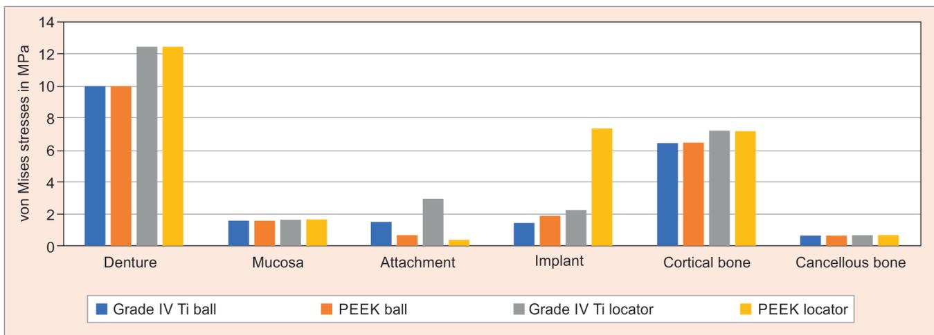
**Fig. 5:** Comparison of VMS generated with the double ball and locator attachments
