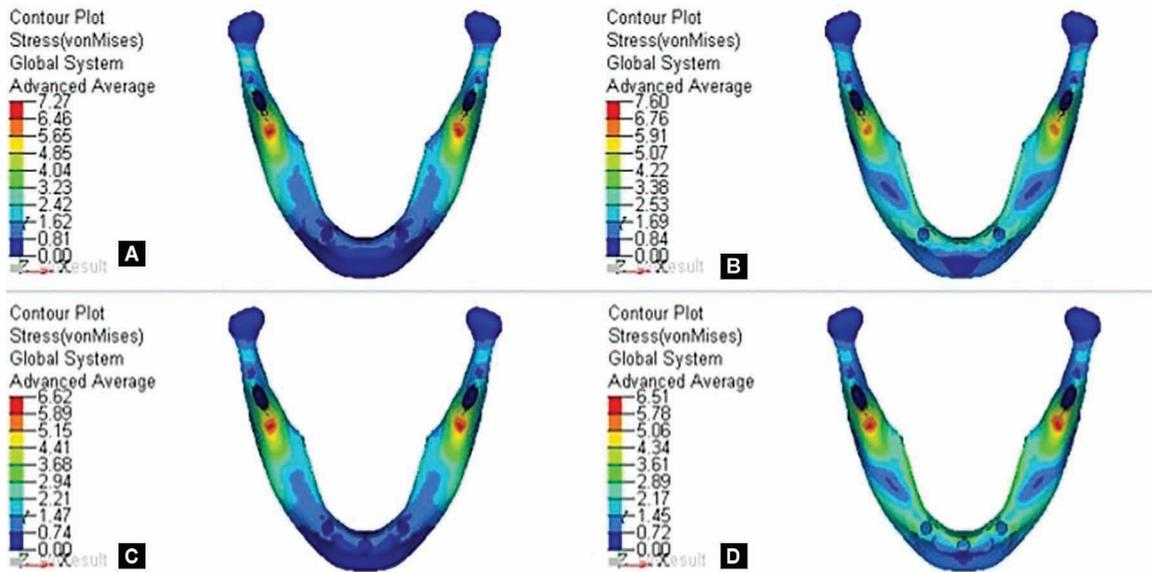
**Figs 4A to D:** Stress in bone distal to implants subjected to two and three locator attachments made of grade IV Ti and PEEK under axial loads; (A) With two locator attachments made of grade IV Ti under axial loading; (B) With two locator attachments made of PEEK under axial loading; (C) With three locator attachments made of grade IV Ti under axial loading; (D) With three locator attachments made of PEEK under axial loading
