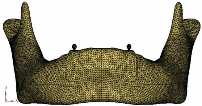
Fig. 1: Meshing of a three-dimensional geometric model of a human edentulous mandible with ball attachments
